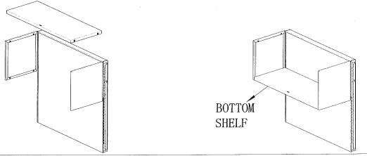
Step 3:Install the door and top shelf together with tapping screws, and then, put it between the shelf ends, finally, tighten all the 8 screw bolts.
