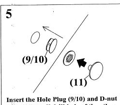
Insert the Hole Plug (9/10) and D-nut Cap (11) to all drill hole of the other edge of Side Panel (C) and Back Panel (B) which the hole are not in use.
